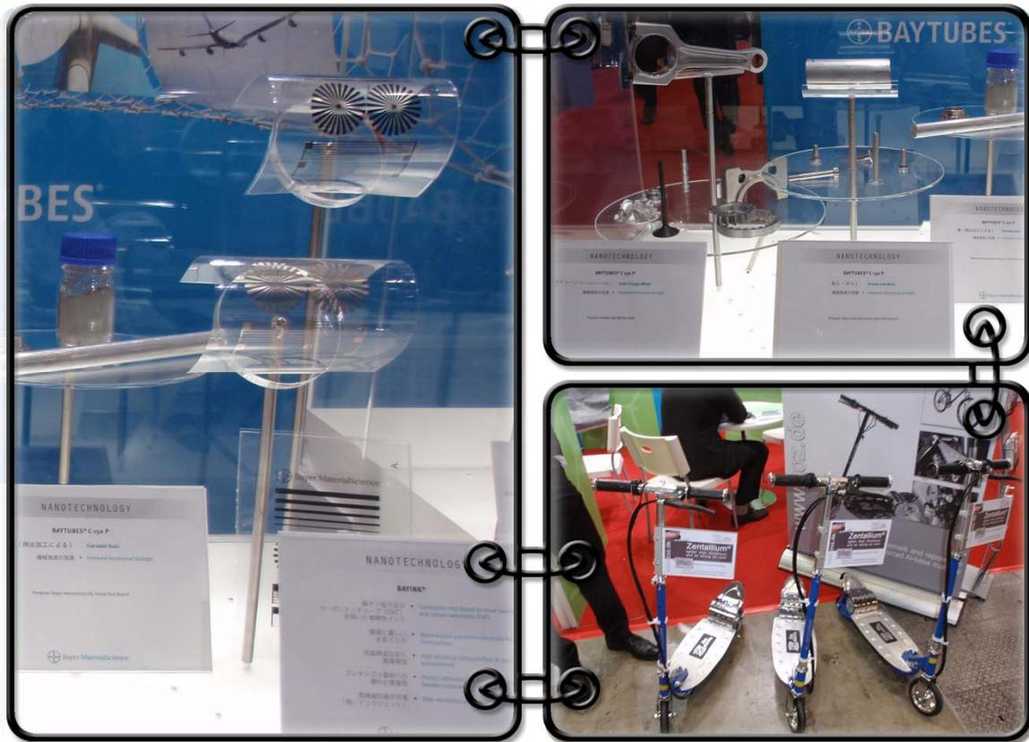
**Fig. 1. Left: BayInk sample and the printed flexible conductive circuits on the transparent substrate; Top right: semi-finished products (rods and complex bars) as well as fasteners (nuts and bolts) made by Bayer CNT-Al composites, which is as strong as steel and as light as Aluminum; Bottom right: Zoz mobility vehicles using Zentallium.**
