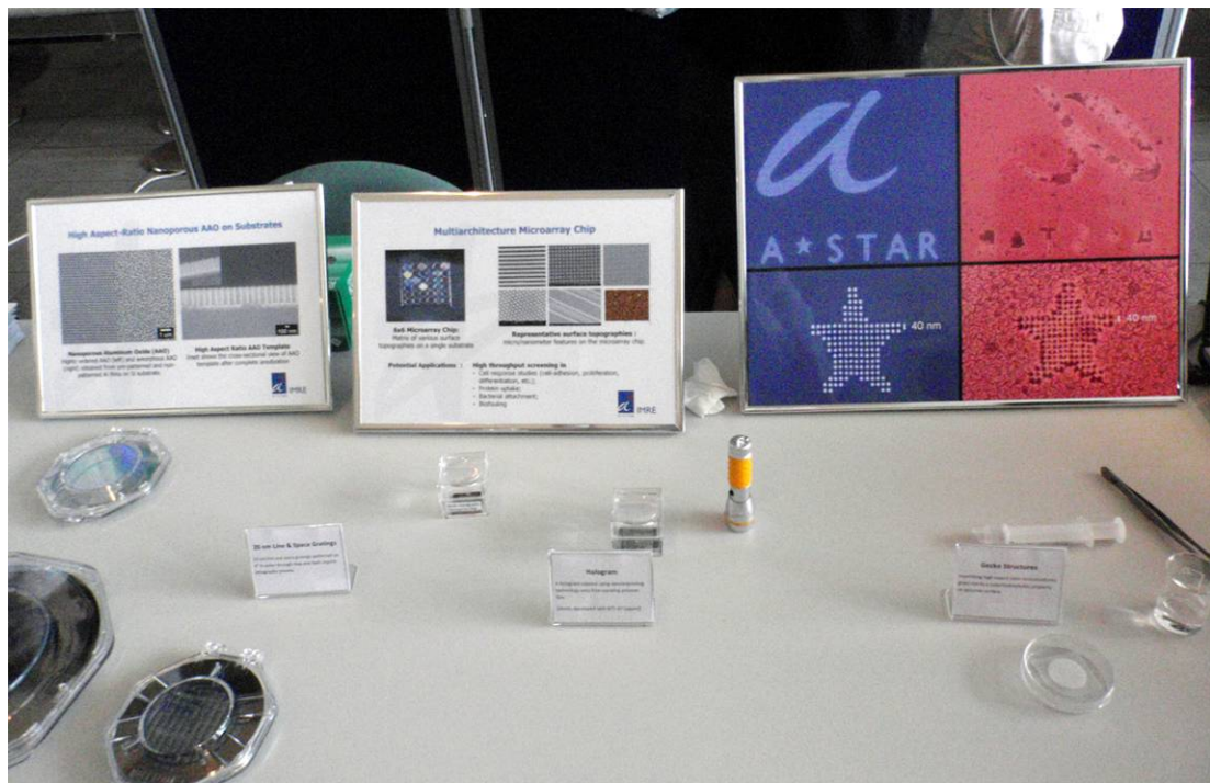
Exhibition of products, produced by the NIL group in IMRE, including gecko structures, hologram surface, 20nm line & space gratings, and high aspect ratio AAO
