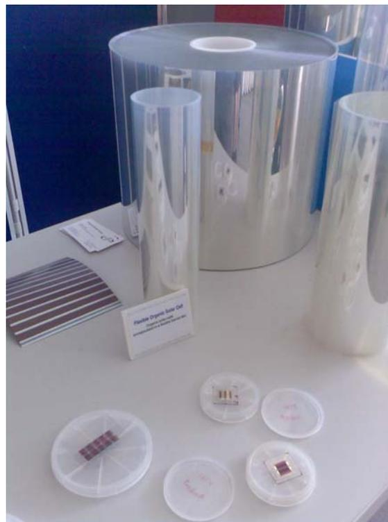
**One example of application: flexible organic solar cell encapsulated in the flexible barrier film**
