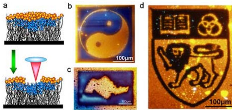
**Fig. 3. (a) Schematic of the patterning process using optical tweezers for quantum dots decorated CNT. Fluorescent microscopy images of (b) Tai Chi pattern (c) Singapore Island (d) NUS logo (Source: Prof Sow CH, NUS)**
