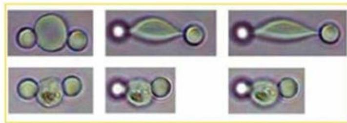
**Fig. 4. Optical tweezers stretching of a healthy red cell (top row) and a stiffer red blood cell in a late stage of malarial infection (bottom row). (Source: Prof CT Lim, Div of Bioengineering, NUS)**
