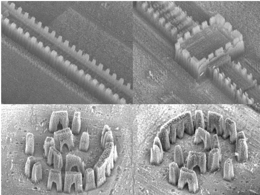
**Fig. 2. Laser pattern CNT into 3D micro-Great Wall and micro-Stonehenge (Source: Prof Sow CH, NUS)**
