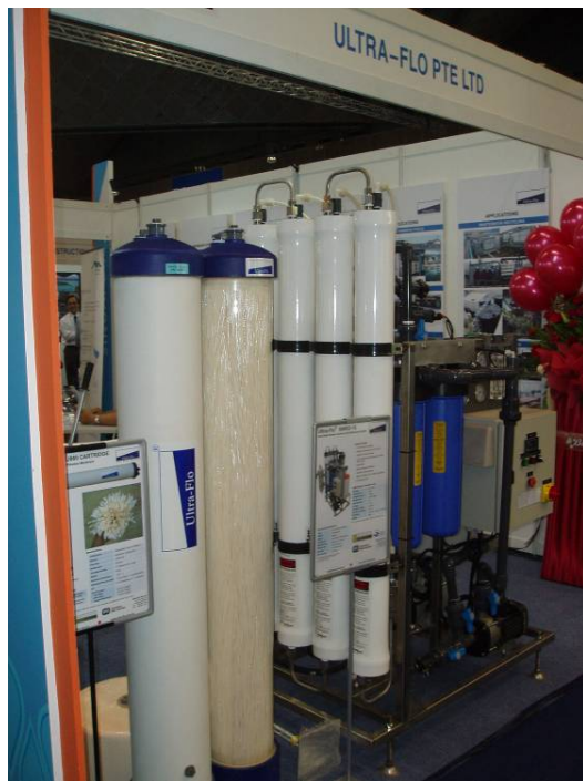
(a) Ultra-Flo's 8-inch ultrafiltration hollow fiber membrane module (b) Toray's 16-inch and 8-inch reverse osmosis membrane elements
