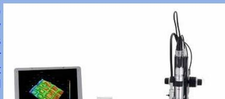
microscope solution. Leica Digital Microscopes do feature outstanding, high-quality optics and also offer a wide variety of quantitative analysis options-whether 2D analyses or advanced 3D surface measurements. The highlights of the DVM series at a glance:
