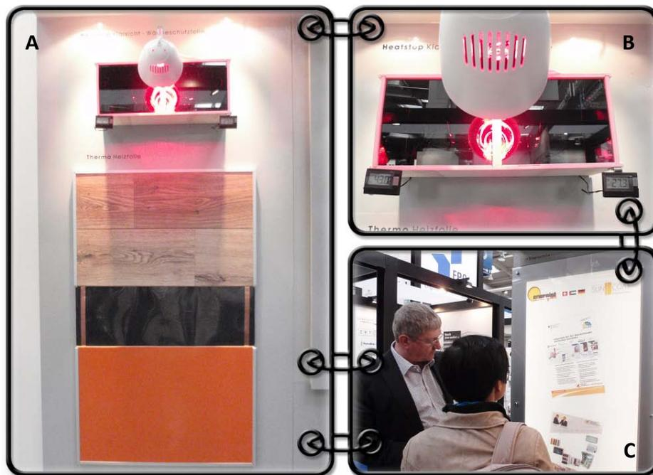
Figure 1. A) SUNCOAT heatstop (top) and thermal heating foils (down) were showcased at Hannover Messe; B) right box covered by SUNCOAT heatstop were always remaining at 27.3 °C while the left box without heatstop protection is heated to 43.7 °C in several minutes; C) Mr Brellos (SUNCOAT) was introducing the partners of SUNCOAT to Dr Lerwen Liu (NanoGlobe) during interview.
