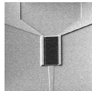
Figure at the right is a Scanning Electron Microscopy (SEM) image of a Ge-on-SOI metal-semiconductor-metal (MSM) photodetector featuring interdigitated grating electrodes for enhanced surface plasmonics effect.
