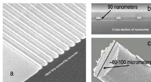
(a) Current nanoTrek® devices consist of 12,000 nanowires ; (b) each nanowire is only 90nm across; (c) which is only ~1/1,000th width of a human hair
