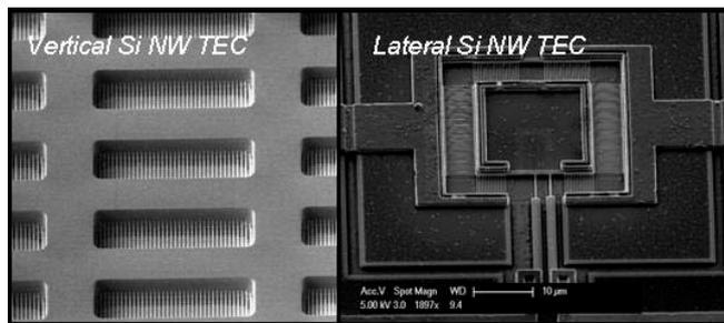
processes are not CMOS compatible. Recent works in IME have suggested that SiNW arrays show great promise as highly scalable and efficient thermoelectric materials. As the dimensions of silicon go below 50 nm, there is a 100 fold decrease in its thermal conductivity (1.6 W/mK) without affecting the Seebeck coefficient or electrical resistivity. This makes SiNW a very promising thermoelectric material because of the low thermal conductivity and established CMOS infrastructure. We
