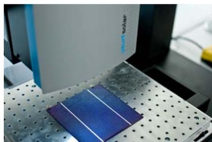
The system is able to conduct up to 12 area measurements within one minute, including procedure time and evaluation. A vacuum chuck guarantees the safe fixture of the solar cell while the high precision x-y stage is in motion. The positioning tables are available up to the meter range, in length and width, which is a necessary feature in measuring entire solar modules.
